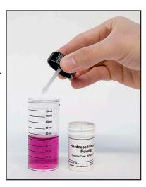
Add Hardness Titrant drop-wise, while swirling, until the sample color changes from red to blue. Record the number of drops.
